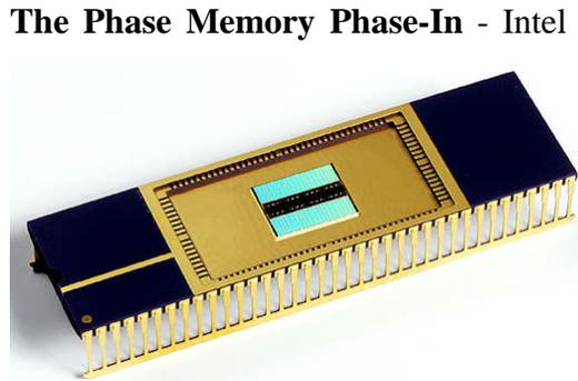
**The Phase Memory Phase-In** - Intel is preparing to sample a 90-nm 128-Mbit phase change memory to customers in the first half of 2007 with mass production before the end of 2007. The memory is a drop-in replacement for NOR flash non-volatile memory although its performance characteristics means it could be used in a greater range of applications and come to replace DRAM in some systems. Intel has been a licensee of chalcogenide-based phase change memory technology from
