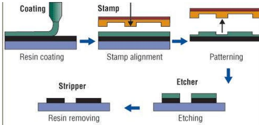
The use of APEM may be able to cut production costs, and here's why. The traditional photolithography process involves the exposure process for patterning that consumes photoresists and developers. But, the imprinting method eliminates the need for the exposure process and only uses the resists to lower material costs. In addition, the simple use of molds for printing, instead of masks, in the exposure process enables huge savings in facility expenditures.
