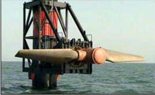
turbine off Devon for four years and plans to install a one-megawatt turbine in Northern Ireland's Strangford Lough this year. Marine Current's design resembles Verdant's but uses two rotors, each with two blades. Other competitors are scaling up so-called ducted turbines, which are surrounded by a power-boosting shroud to guide water flow. Nova Scotia Power recently signed up Dublin's OpenHydro to install a 1-Megawatt ducted
