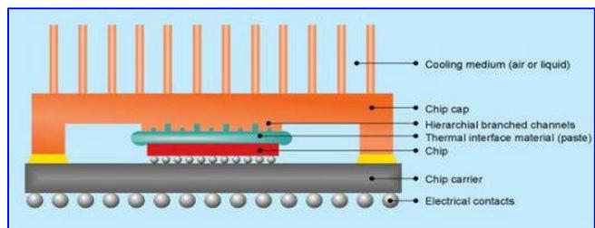
twofold increase in cooling performance. The micrometer-sized channels basically act as an "irrigation system" to allow the toasty particles to homogeneously escape rather than building up in the self-proclaimed "magic cross" section. [*Breakthrough? A real stretch.*]
