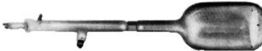
Figure 1 – 1897 Braun Tube – Early Hermetic Package
