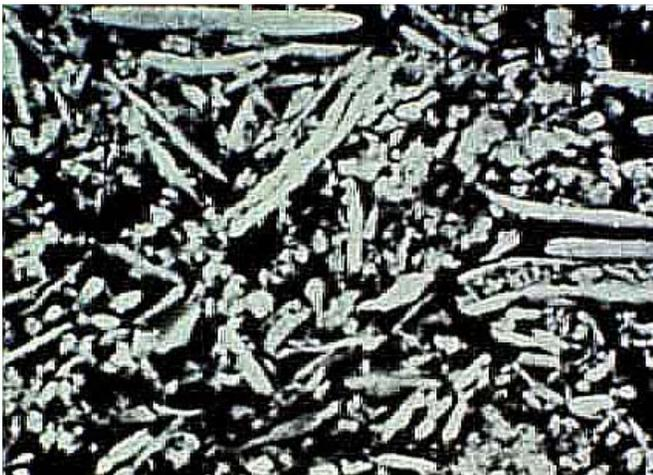
Figure 1 – Conductive Adhesive SEM
