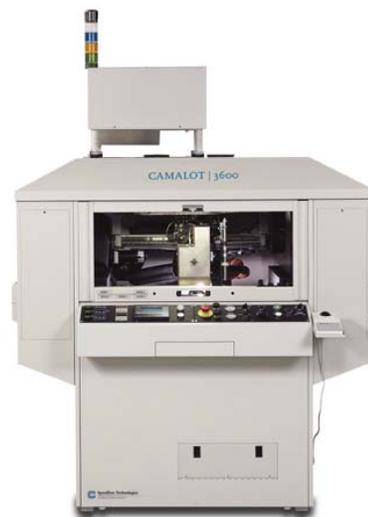
Figure 10 – Needle Dispenser (Speedline/Camalot)
