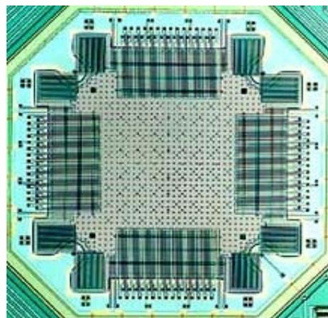
Figure 1 – Accelerometer - ADI
