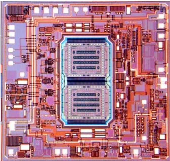
Figure 2 – Gyroscope - ADI
