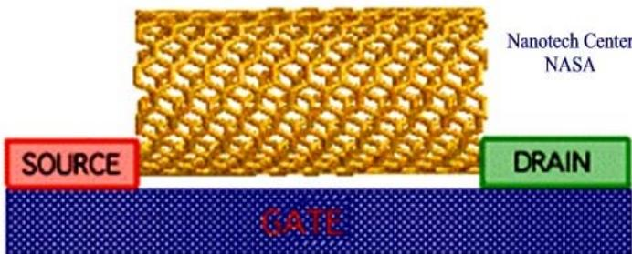
Figure 13 – CNT Transistor Diagram - NASA
