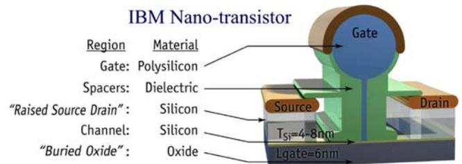
Figure 16 – Nano Si Device - IBM
