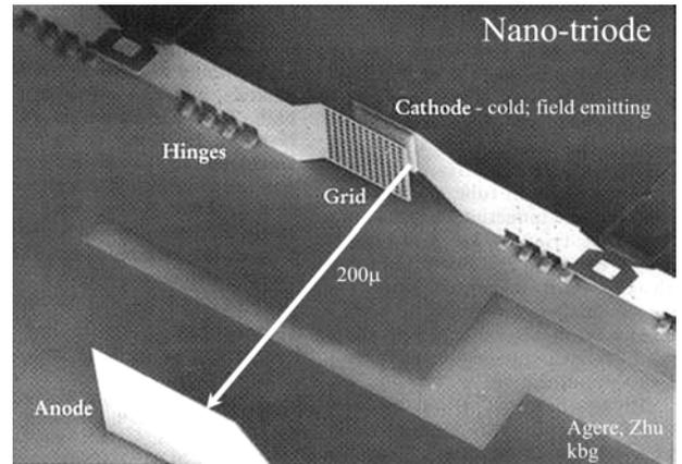
Figure 15 – IBM CNT Triode – AT&T
