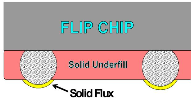
Figure 8 – Type 2 Flux/Underfill
