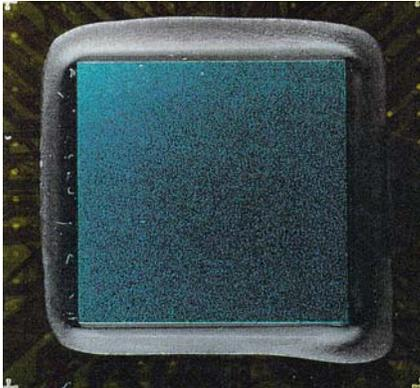
**Figure 2 - Pentium II Flip Chip** - Prismark
