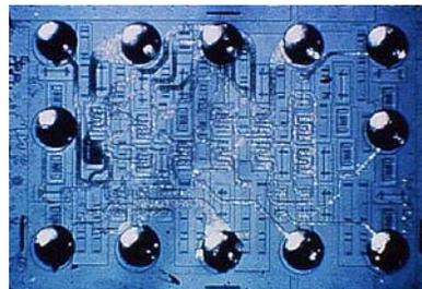
Figure 1: 1<sup>st</sup> Generation FC – IBM
