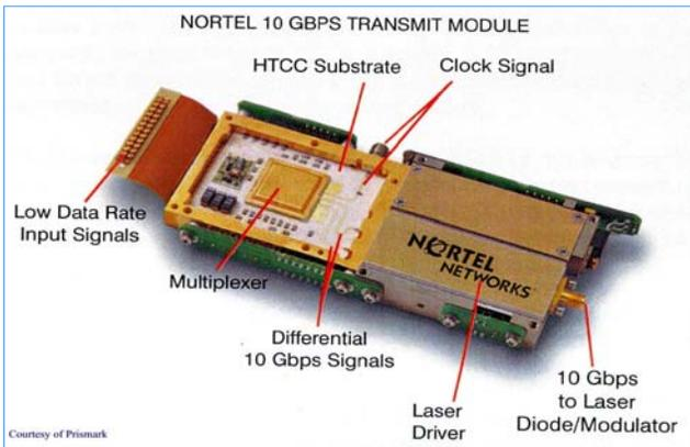
Figure 3 – Laser Transmitter– Nortel Networks
