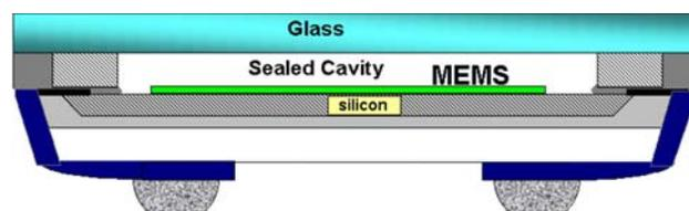
Figure 12 – OE CSP - Shellcase
