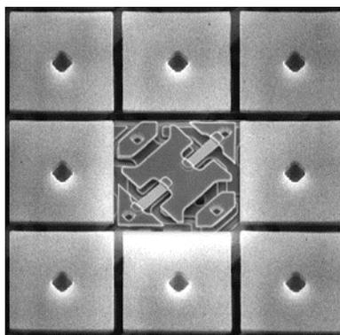
Figure 9 – Micro-Mirror MOEMS Chip – Texas Instruments (The center mirror is removed to see the internal structure)
