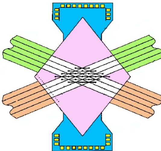
Figure 10 – MOEMS Bubble Switch (Agilent)
