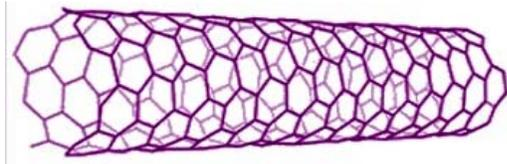
CNT Structure (each connection point is a carbon atom)
