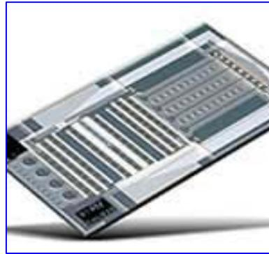
A researcher mixes a DNA sample with a polymerase enzyme and DNA primers and passes it through a bank of 12 microscopic channels, each measuring 150 - 200 microns, within the silicon. Electrical heating elements that are embedded resistors
