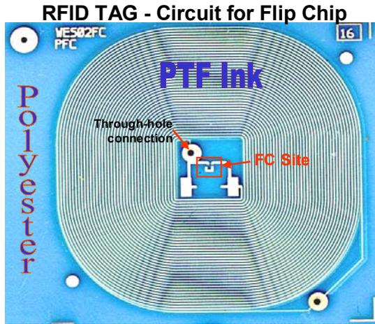
Figure 4 – RFID Antenna
