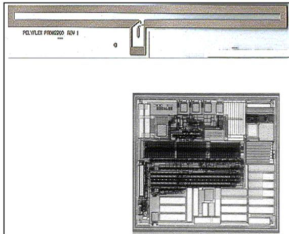
Figure 5 - RFID Flip Chip & Antenna Circuit
