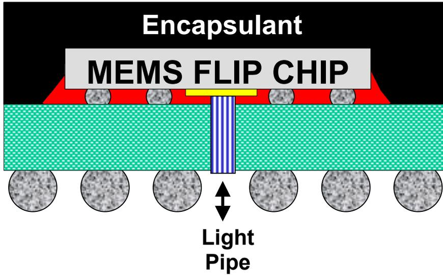
Figure 6 – Flip Chip In Package MOEMS
