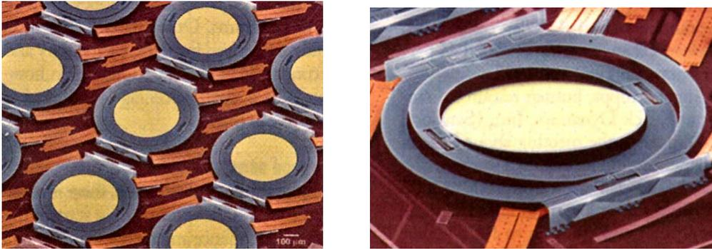
**Figure 2 – Lamda Router Mirror Switch – Lucent**
