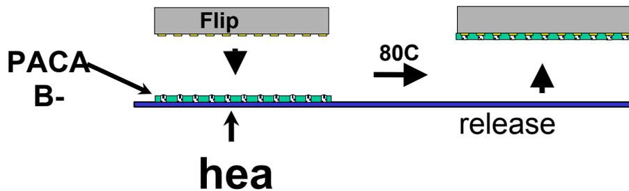
2. Assembly: Flip Chip to substrate (full bond)
